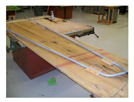
OK, notice in the pic above right that I bent the front of the conduit so that the pieces will come together at the front. They will be positioned so that they come together and also turn slightly upward.
