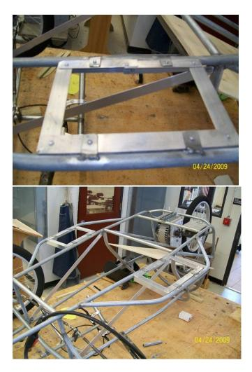
Because of the weight of the batteries, the bottoms of the side pods need additional support along the outside. In this case I used 1/8" steel round stock (welding rod) to make a pair of diagonal struts for each battery pod. The forward ones are welded to the outer bottom rail in front of the battery tray and to the top rail near the steering wheel crossmember. The rear ones are welded to the outer bottom rail behind the battery tray and to the main roll cage hoop.
