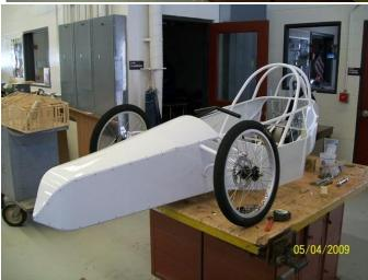
The cowl piece was next. This turned out to be one of the most tedious pieces to make. I cut and re-cut the pattern several times before I got it to fit correctly. I wanted it to rise or flare upward so that it would be above the driver's hands on the steering wheel, but not so high that it would obscure forward vision. Also, the trailing edge had to be rolled for strength and safety.
